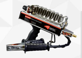
BLT600S is a device for testing 6V and 12V starter batteries. The tester simulates the battery load through a set of load resistors. Their selection allows you to adjust the load in accordance with the characteristics of the tested battery. The clear display allows you to present voltage changes during measurement.
